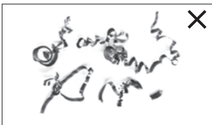
Apple-peel-like chips (Without curling)
