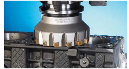
Roughing for cast iron
