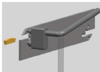
② Clamp the insert on its seat after turning the handle to 45°~160° for loosening the seat.
