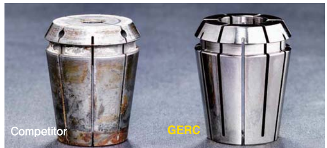
Two samples of collets after 4 months of use : Left : Non-coated, Right : GERC collet
