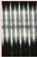
Screw Thread pitch= 0.5mm
