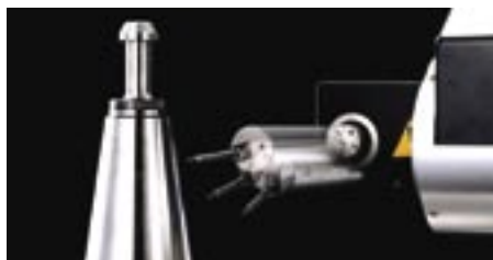
Detector rotation mechanism (0 to 290°, in increments of 1°)
