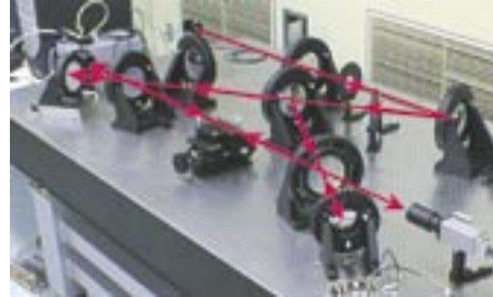
double-faced interferometer (DFI)
