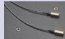
Temperature compensation system (photo: temperature sensors)
