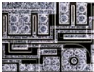
Dark field (DF) observation: Observing only the scattered light by shutting down the direct light to the objectives. The scratches and dust that cannot be viewed in the bright view field can be observed by a high-contrast.
