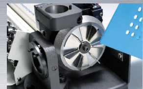
CBN diamond grinding wheel assures extra fine sharpening effect.
