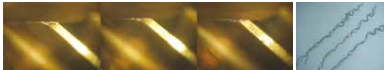
Competitor A(Total Tapping 490 Holes)-Thread
