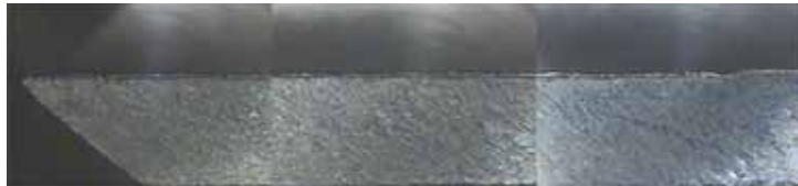
YG-1 (Total Milling Length 100m)
