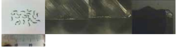
COMPETITOR A (Total Milling Length : 25m)
