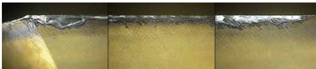
COMPETITOR A (Total Milling Length : 60m)
