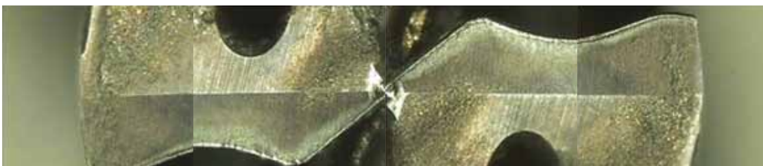
COMPETITOR A (After Drilling 546 Holes)
